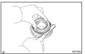
Using a feeler gauge, measure the clearance between the synchronizer ring back and gear spline end.
