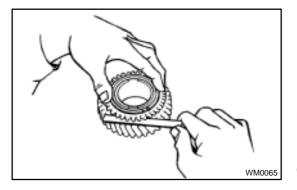
(d) Using a feeler gauge, measure the clearance between the synchronizer ring back and gear spline end.
